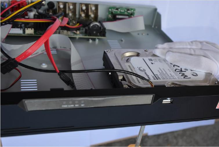
Step 4 Turn the device over, and fasten the rest two hard disk fixing screws, as shown in Figure 2-3.
